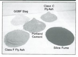
has cementitious properties by itself but these are enhanced when it is used with portland cement. Slag is used at 20% to 70% by mass of the cementitious materials.
