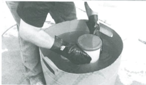
Making and Curing Cylinders in the Field
